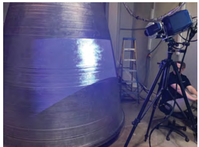
DM3D used Hexagon measurement technologies to prove that it could meet NASA's tolerance requirements in producing a full-scale NASA RS-25 nozzle liner.
